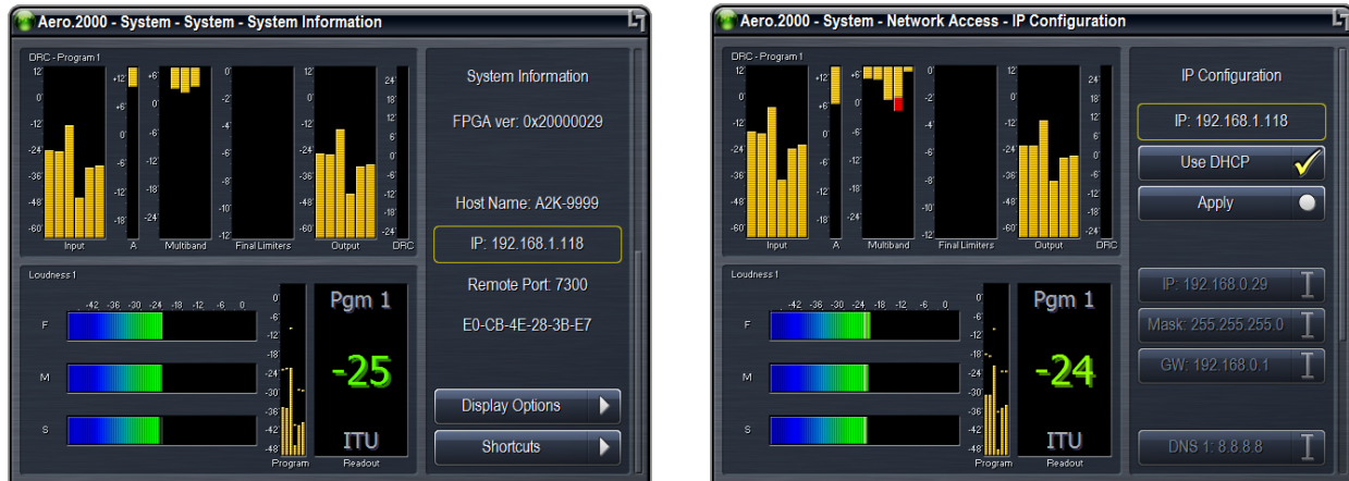
Figure 1-10 Left: IP address, remote port, and MAC address; Right: reconfiguring IP settings
