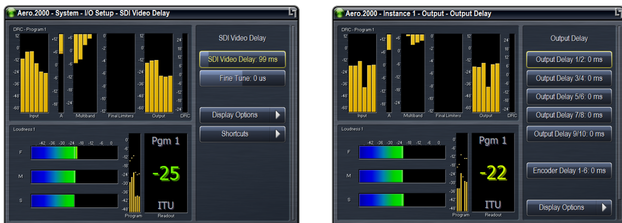
Figure 1-11 Left: SDI video delay settings; Right: Output Delay settings available for each instance
